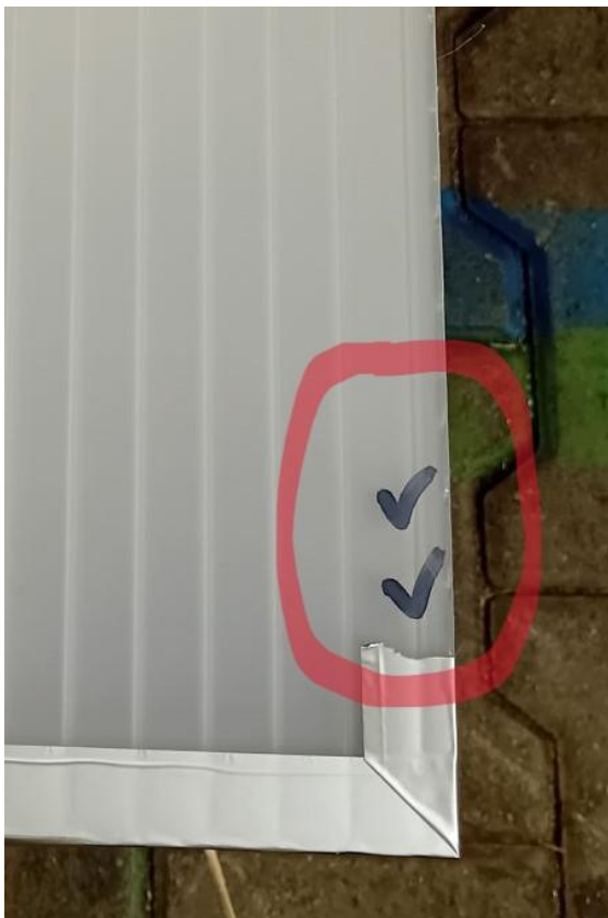
Figure 45 Method of marking the UV-resistant side of polycarbonate sheets.
